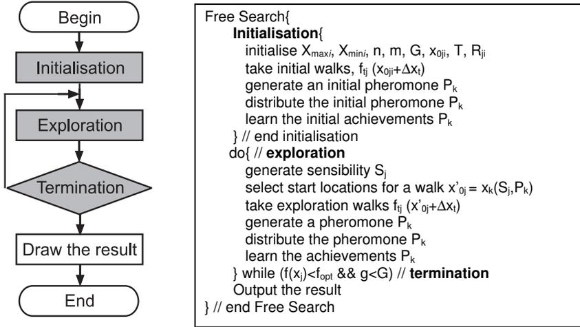
Figure 1. Free Search – algorithm architecture and an example in pseudo code.
