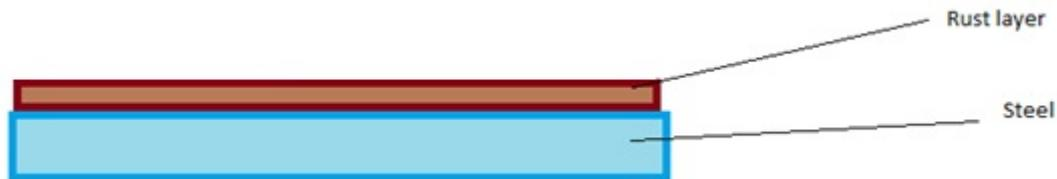
**Figure 2: Diagrammatic representation of surface rust on steel**
