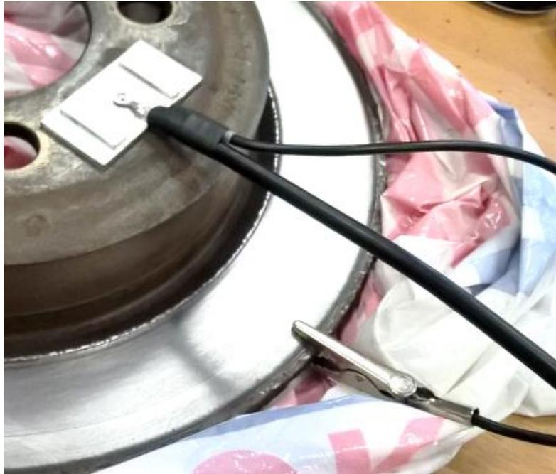
Figure 10: Brake disc showing sensor on area 1 and ground clip placement
