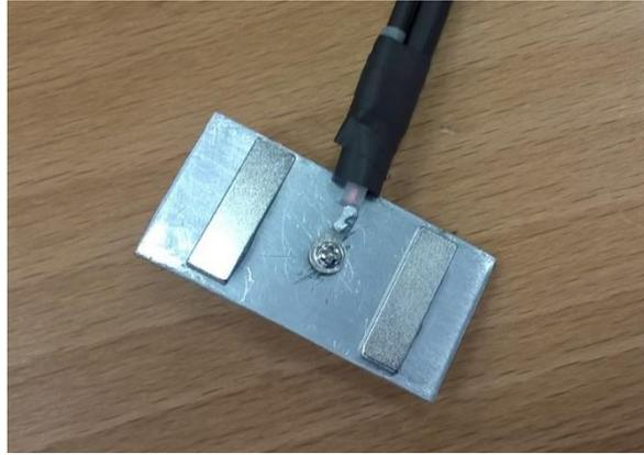
**Figure 7: Practical realisation of Al and Nd sensor**
